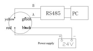
1.Please note that the cable should be correctly connected with reference to the wiring diagram, such as the use of shielded cable The shielding layer should be connected to the shielding ground and ensure reliable connection.
